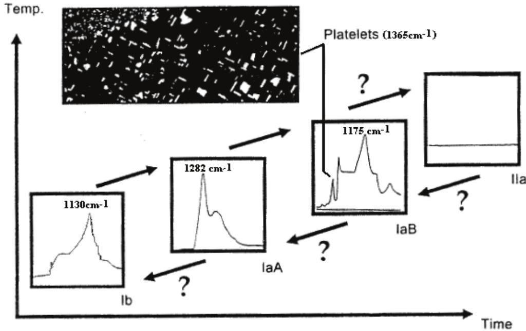
Figure 2 - Temperature versus time schematic representation of the evolution of nitrogen aggregation from C centres (Ib diamonds) to A (IaA diamonds) and B centres (IaB diamonds). Platelets seem to appear during A to B centres transformation. Squares show the infrared absorption envelopes corresponding to each nitrogen aggregation state (modified from Mendelsohn & Milledge, 1995).
