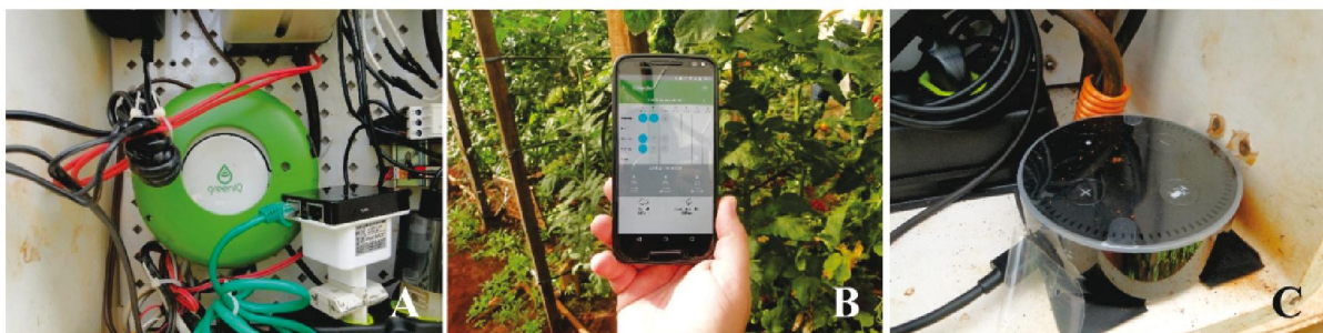
Figure 3 - A) Equipment used: GreenIQ® controller; B) Graphical interface of the soil irrigation management application and C) Alexa® personal assistant from Amazon® (SOUZA; CONCHESQUI; SILVA, 2019)
