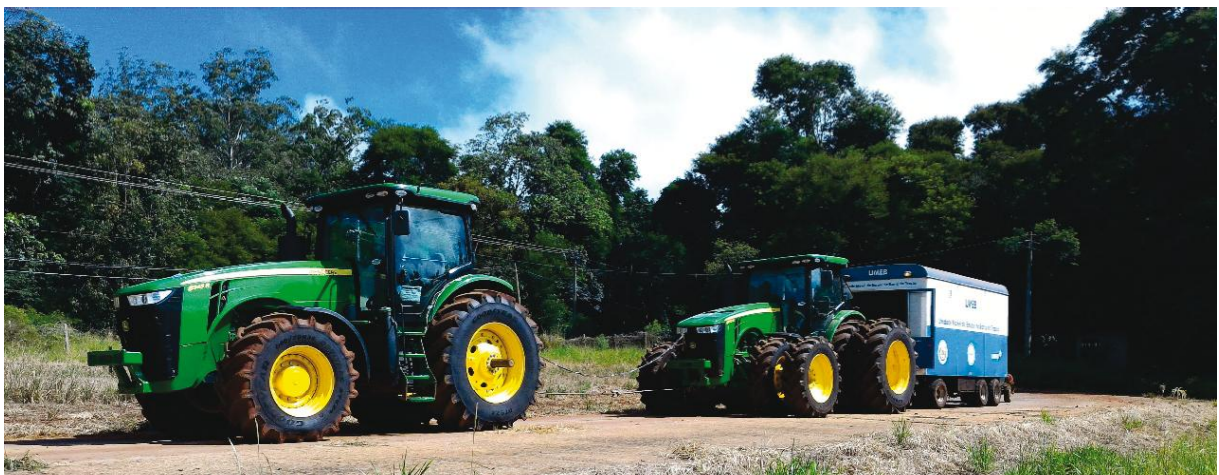
Figure 3 - Dynamometer unit for the application of controlled loads in drawbar performance tests. NEMPA/Botucatu 2018
