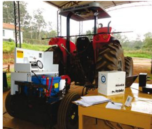
Figure 1 - Dynamometer test of an agricultural tractor, work bench, and instrumentation. NEMPA/Botucatu 2017
