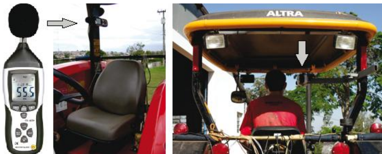
Figure 6 - Instrumentation for testing noise in an agricultural tractor
