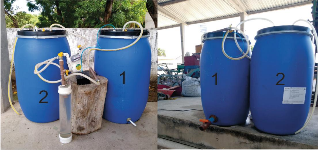
Figure 4 - Small-scale biodigester prototype (for evaluation), in the experimental area of the Department of Agricultural Engineering
