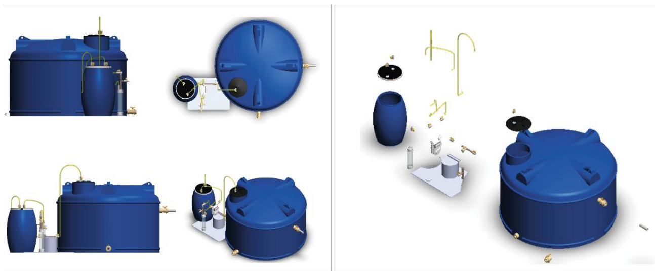
Figure 5 - Representation of the conceptual design of the full-scale biodigester
