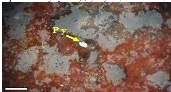
Figure 4 - The higher values of iron oxides have led to a red matrix (probably due to the presence of jasperoid) (Py: Pyrite, scale: 2 mm)
