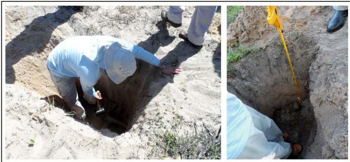
Figure 5 - Field sampling procedures for OSL dating.
