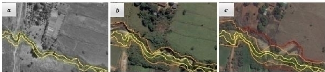
Figure 8 - Situation of a segment with a low altimetric gradient of the drainage channel in 1992 ( a ); 2005 ( b ), and 2016 ( c ).
