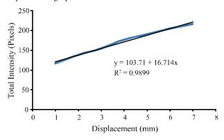
**Figure 7 -** Pixel intensity variation versus diaphragm element displacement graph for the trial 2
