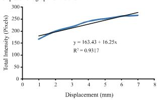
**Figure 8 -** Pixel intensity variation versus diaphragm element displacement graph for the trial 3
