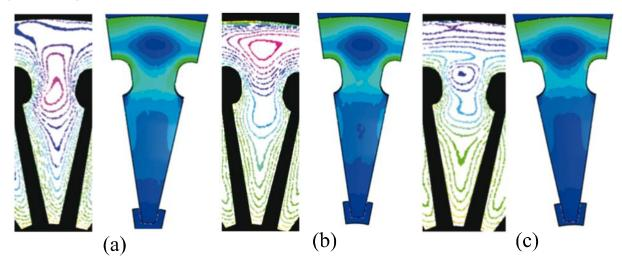
However, such a geometrical differentiation generates certain variations on the stress distribution during loading. That hypothesis was verified by means of the extensometric technique.
