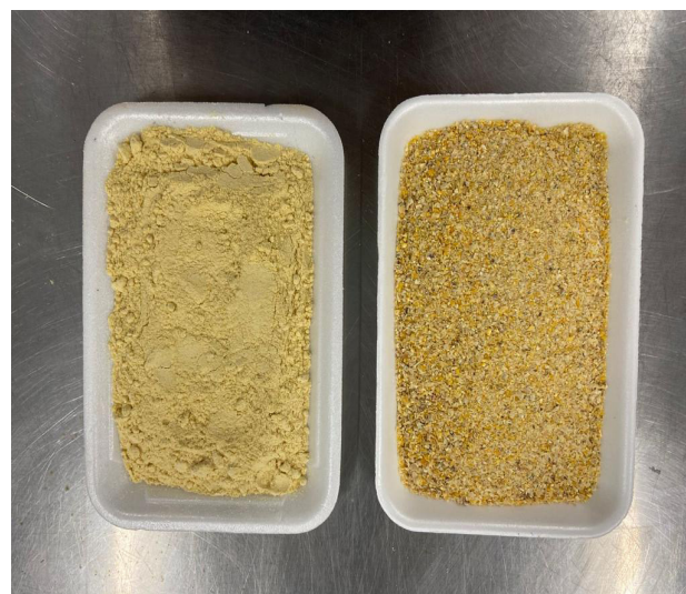
Figure 2 - Raw bran from corn degermination (left side) and flour obtained by sieving (right side)
